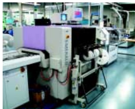
2000 Capacity increased further by a new SMD production line with a vapour-phase soldering system that reduces component stress
