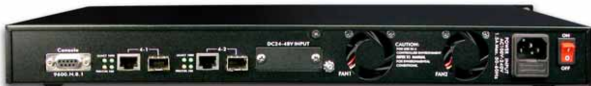
Fig. 2: Access Switch Fast Ethernet backside
