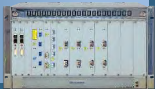
Carrier class chassis 6U 19", 6U, 19 module slots
